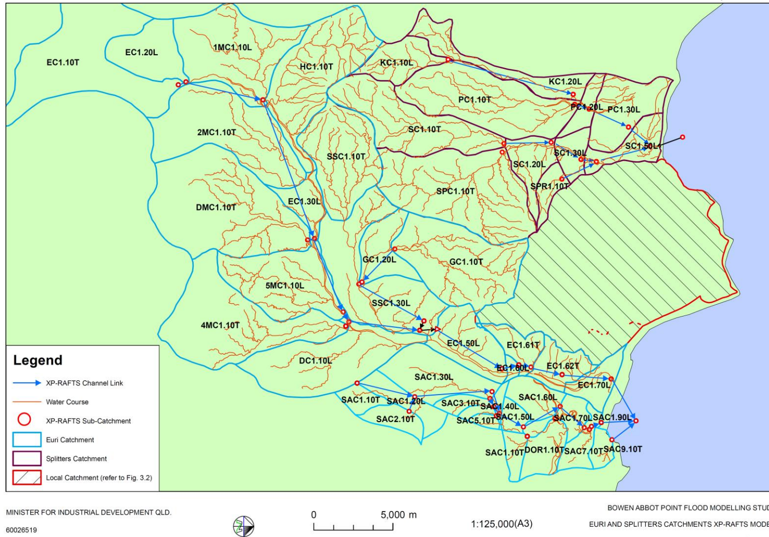
Figure A-1 XP-RAFTS Model Configuration – Euri Creek and Splitters Creek Catchments (Source: Maunsell, 2008)
