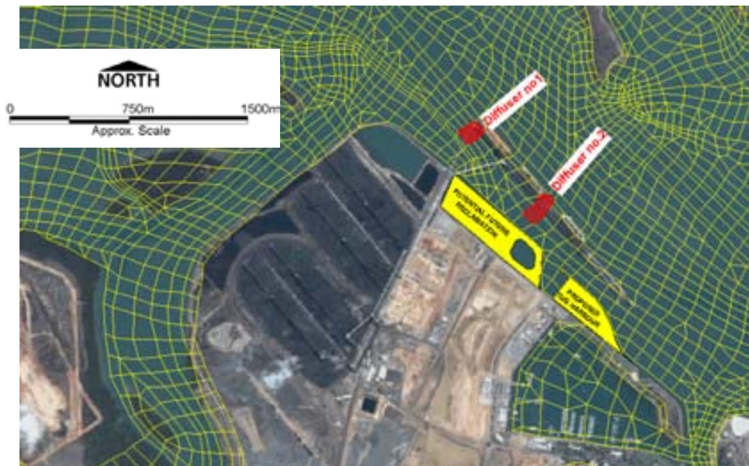
Figure 6-1 Model Elements Selected to Represent Diffuser Lines. Stage 1 Employed Diffuser 1 Only, and Stage 2 Employed both Diffusers
