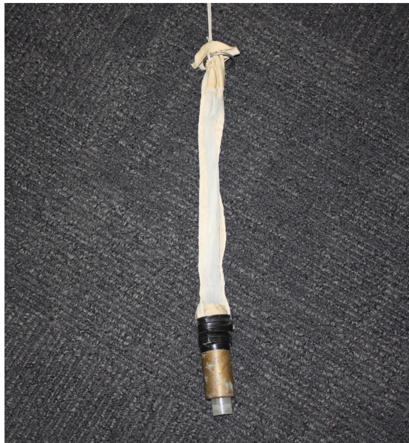
Figure 2 Example of a net used to sample stygofauna, with collection vial attached to bottom of net
