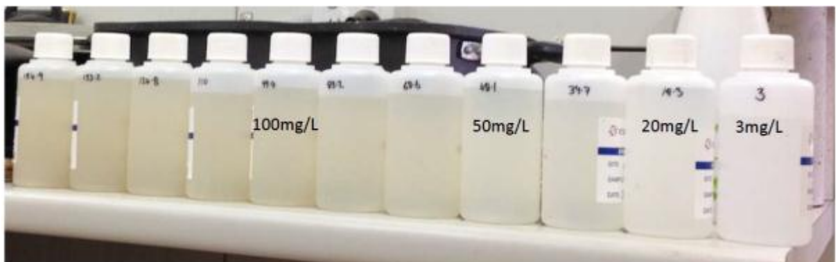
Figure 6-1 Examples of a range of TSS concentrations (photo courtesy of RHDHV)
