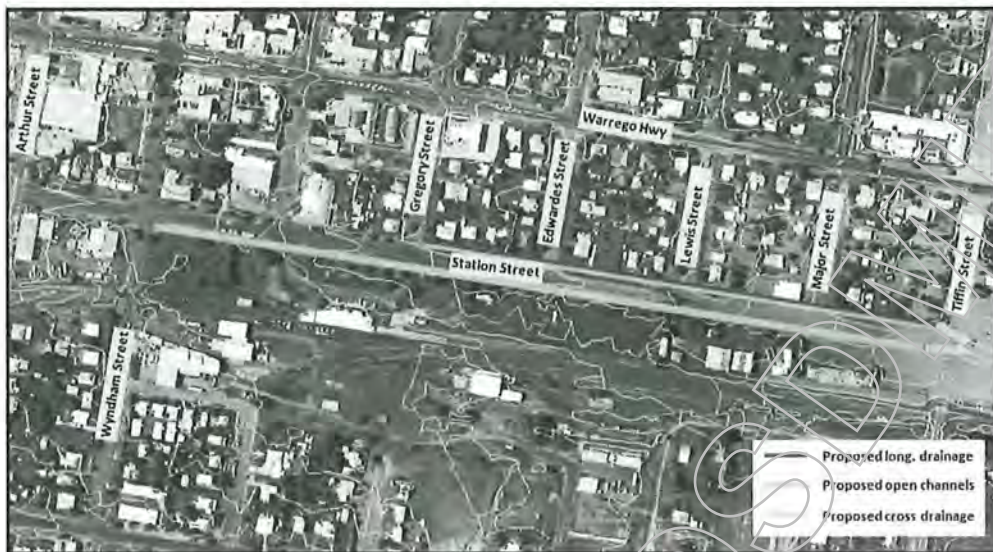
Figure 8-8 Proposed drainage system at Station Street
