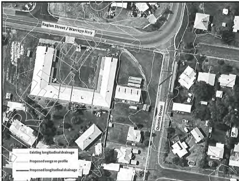
Figure 8-16 Proposed drainage system at Quintin Street
