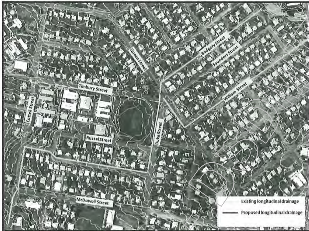
Figure 8-14 Proposed drainage system at Saunders Street
