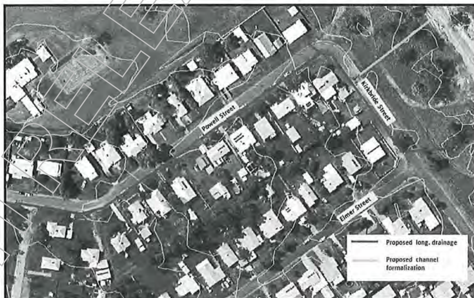
Figure 8-5 Proposed drainage system at Powell and Kirkbride Streets
