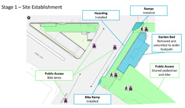
Figure 4.1 Construction Stage 1 - Site Establishment
