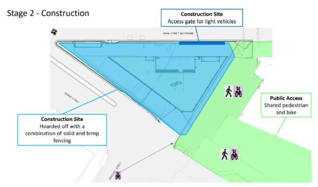
Figure 4.2 Construction Stage 2 - Construction
