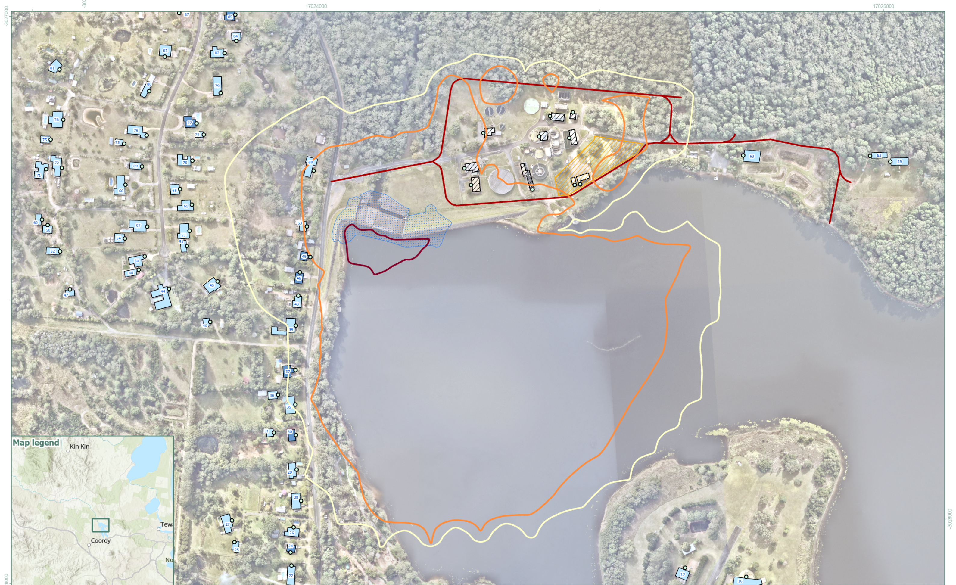
Figure 8 - Lake Macdonald CNVIA - CS6 - Dam Construction Building details include: a reference number, usage and the highest calculated noise level Work activity location: Dam construction area Noise contours: facade corrected modelled at 1.8m height - LAeq dB(A) Lake Macdonald CNVIA
