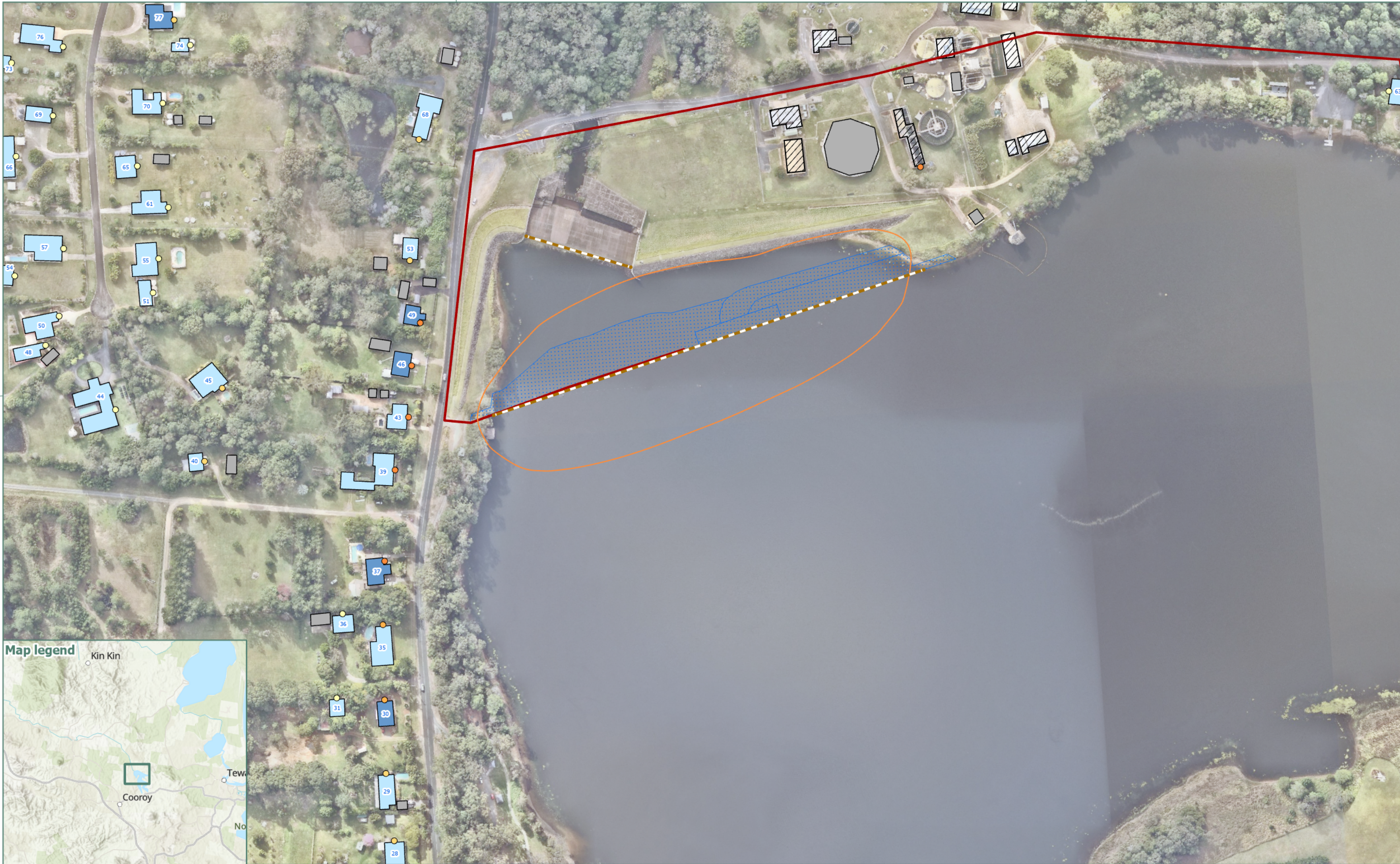
Figure 5 A - Lake Macdonald CNVIA - CS3A - Cofferdam vibratory sheet piling
