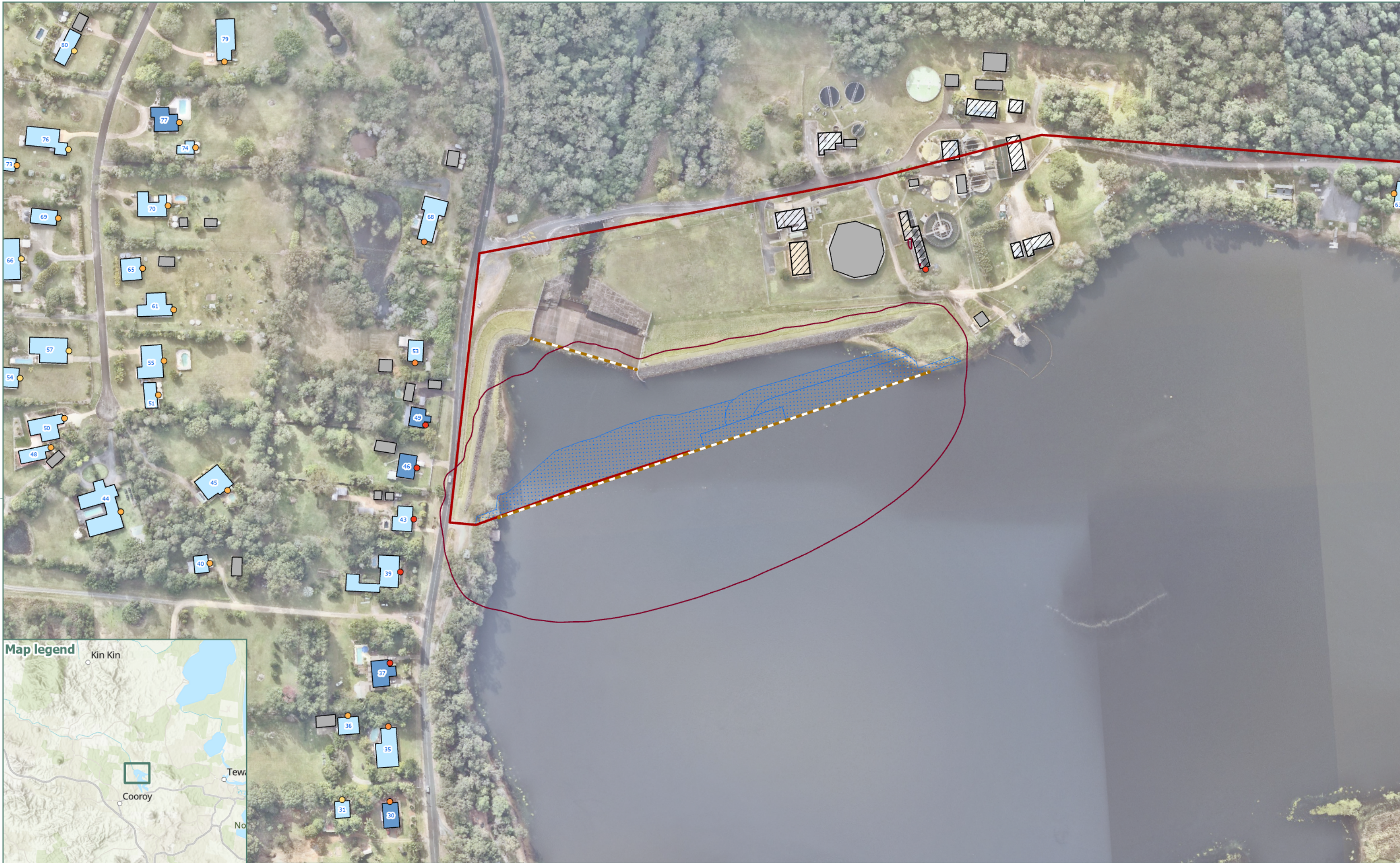
Figure 5 B - Lake Macdonald CNVIA - CS3B - Cofferdam impact sheet piling Building details include: a reference number, usage and the highest calculated noise noise level Work activity location: Impact piling Location & Lorry Route Noise contours: facade corrected modelled at 1.8m height - LAeq dB(A) Lake Macdonald CNVIA
