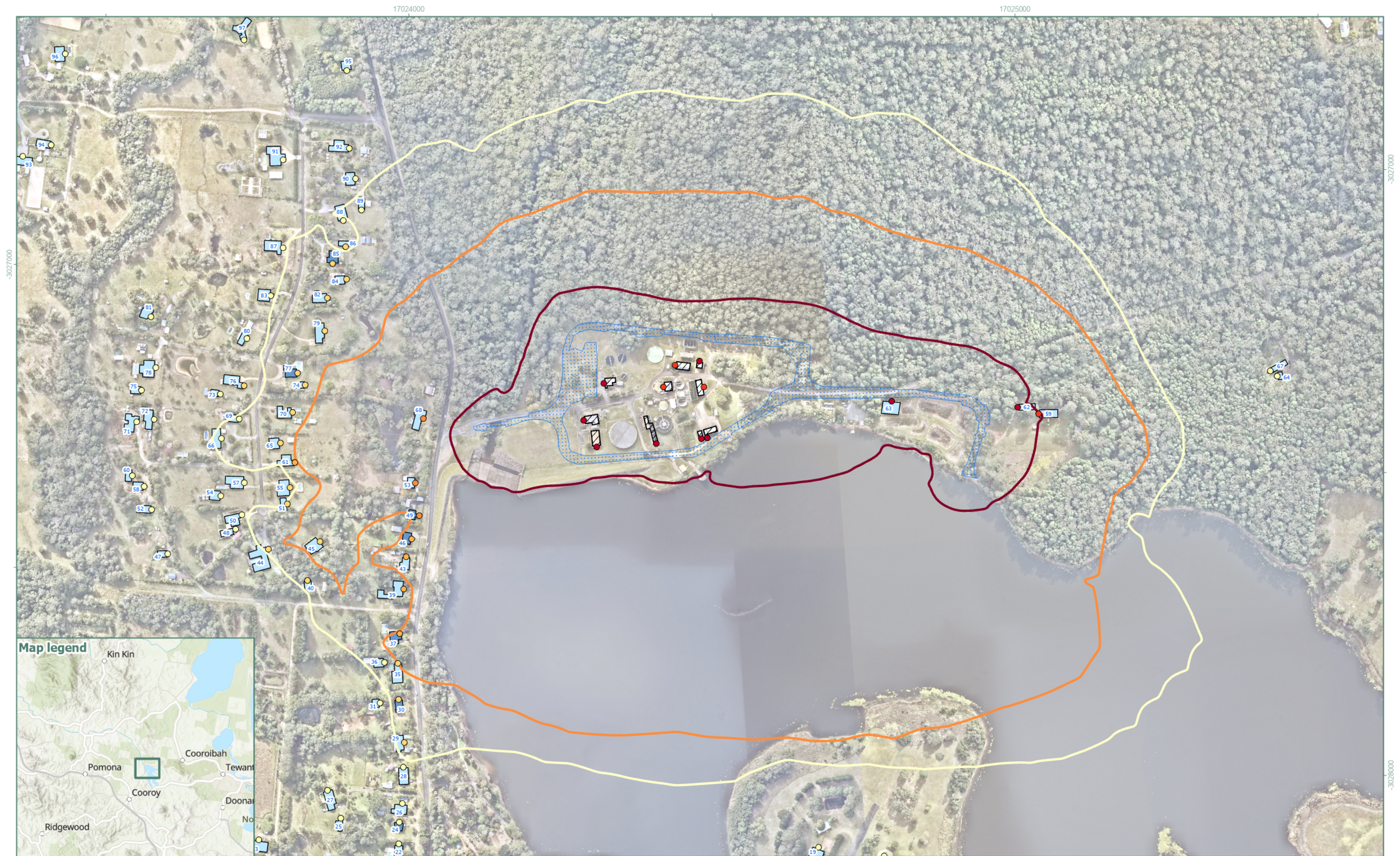
Figure 4 - Lake Macdonald CNVIA - CS2 - Site gravel road construction Building details include: a reference number, usage and the highest calculated noise level Work activity location: Road and carpark construction area Noise contours: facade corrected modelled at 1.8m height - LAeq dB(A) Lake Macdonald CNVIA
