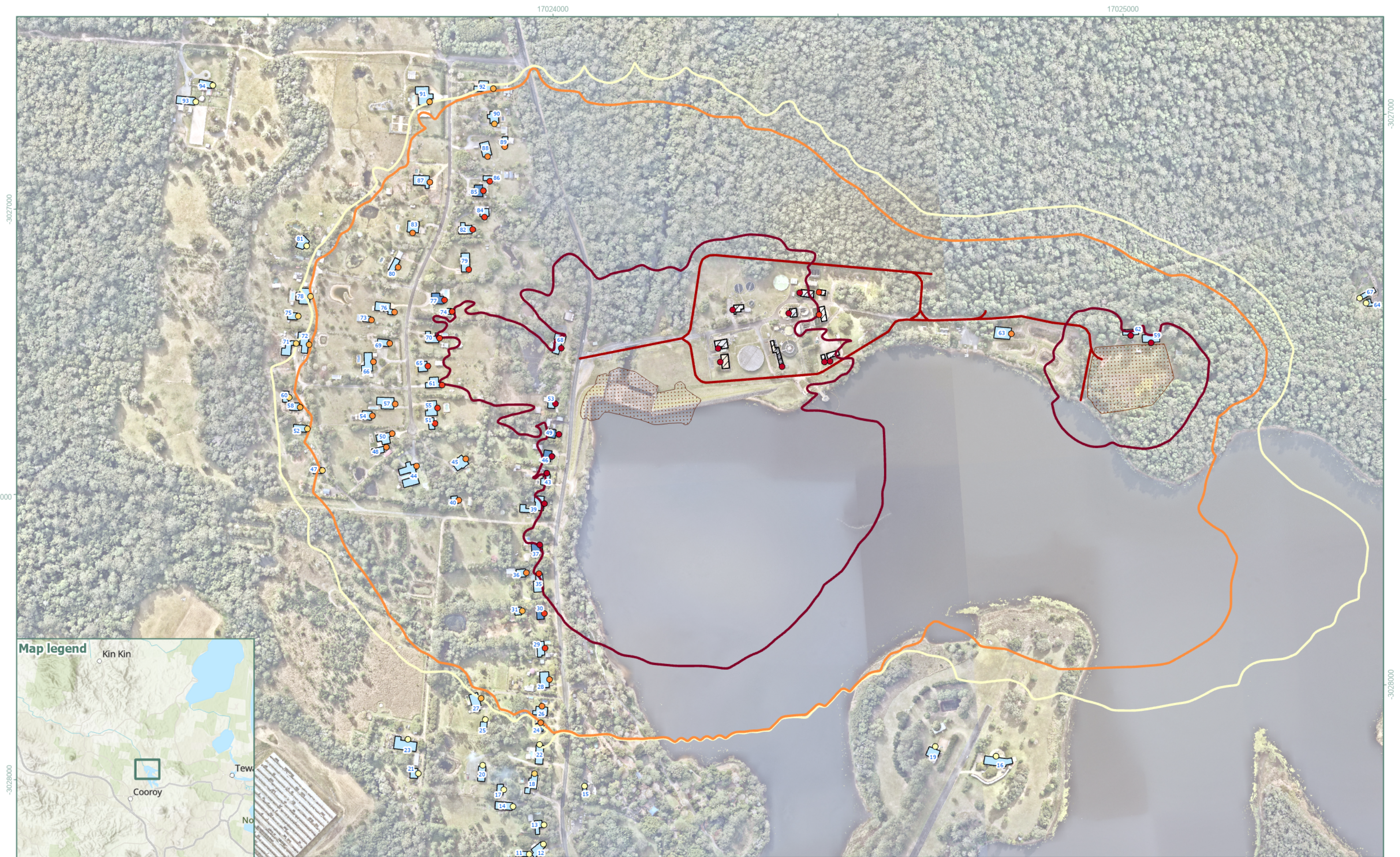
Figure 7 - Lake Macdonald CNVIA - CS5A & 5B Dam Crest and spillway demolition Building details include: a reference number, usage and the highest calculated noise level Work activity location: Spillway demolition and excavation area Noise contours: facade corrected modelled at 1.8m height - LAeq dB(A) Lake Macdonald CNVIA
