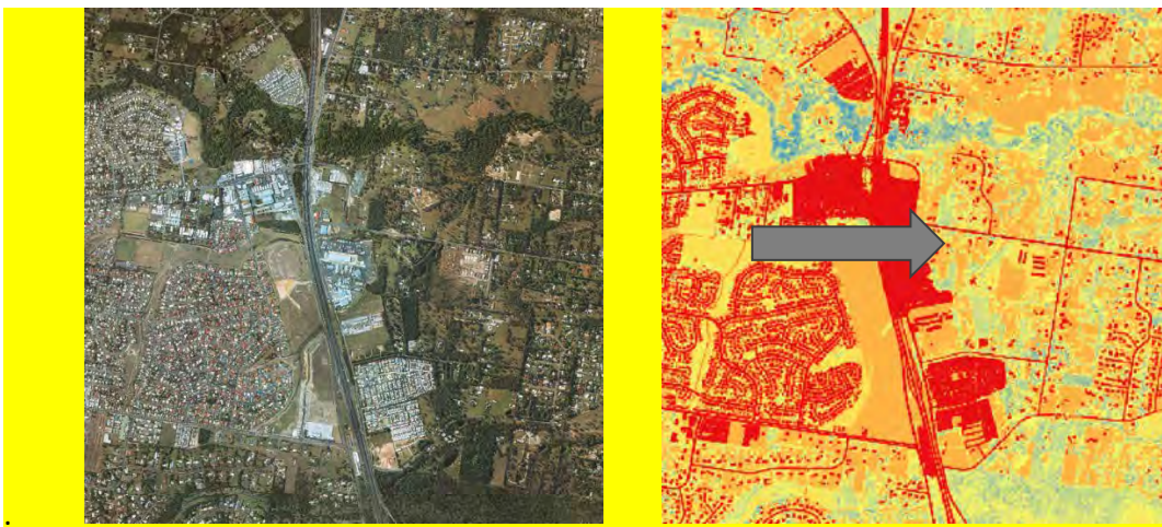
Remote sensing shows the potential for urban heat island effect red = high/hot, blue = low/cool
