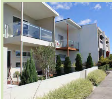
(Maroochydhore) The front door and pedestrian entry as well as habitable room windows should face all primary frontages (whether streets or public open space).
