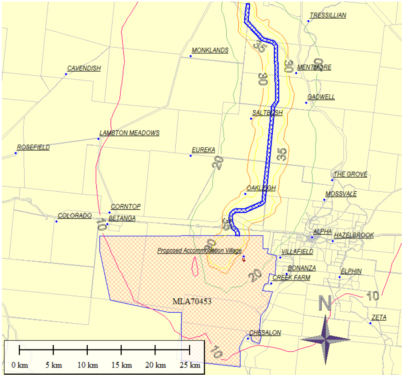
Figure 16: Calculated Maximum Noise Levels from Railway Locomotives [dB(A)]
