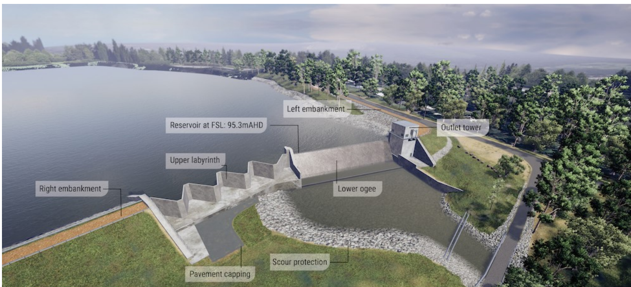
Figure 3-1: Proposed Dam Upgrades
