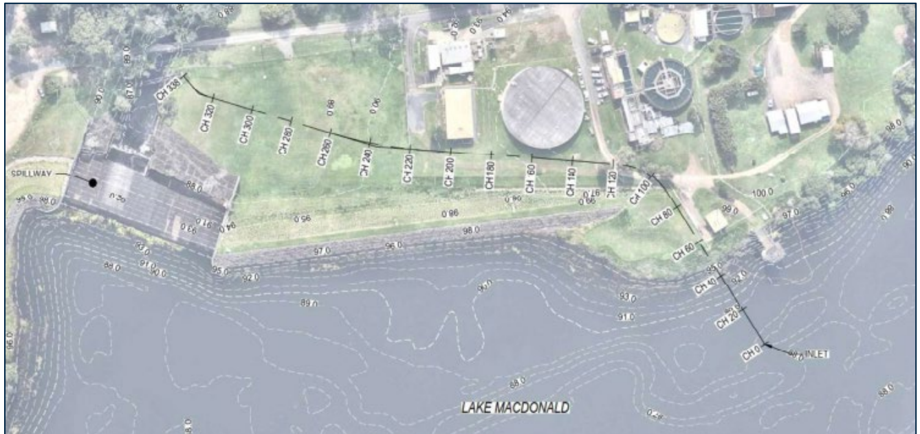
Figure 15: Proposed alignment for the pump & siphon system
