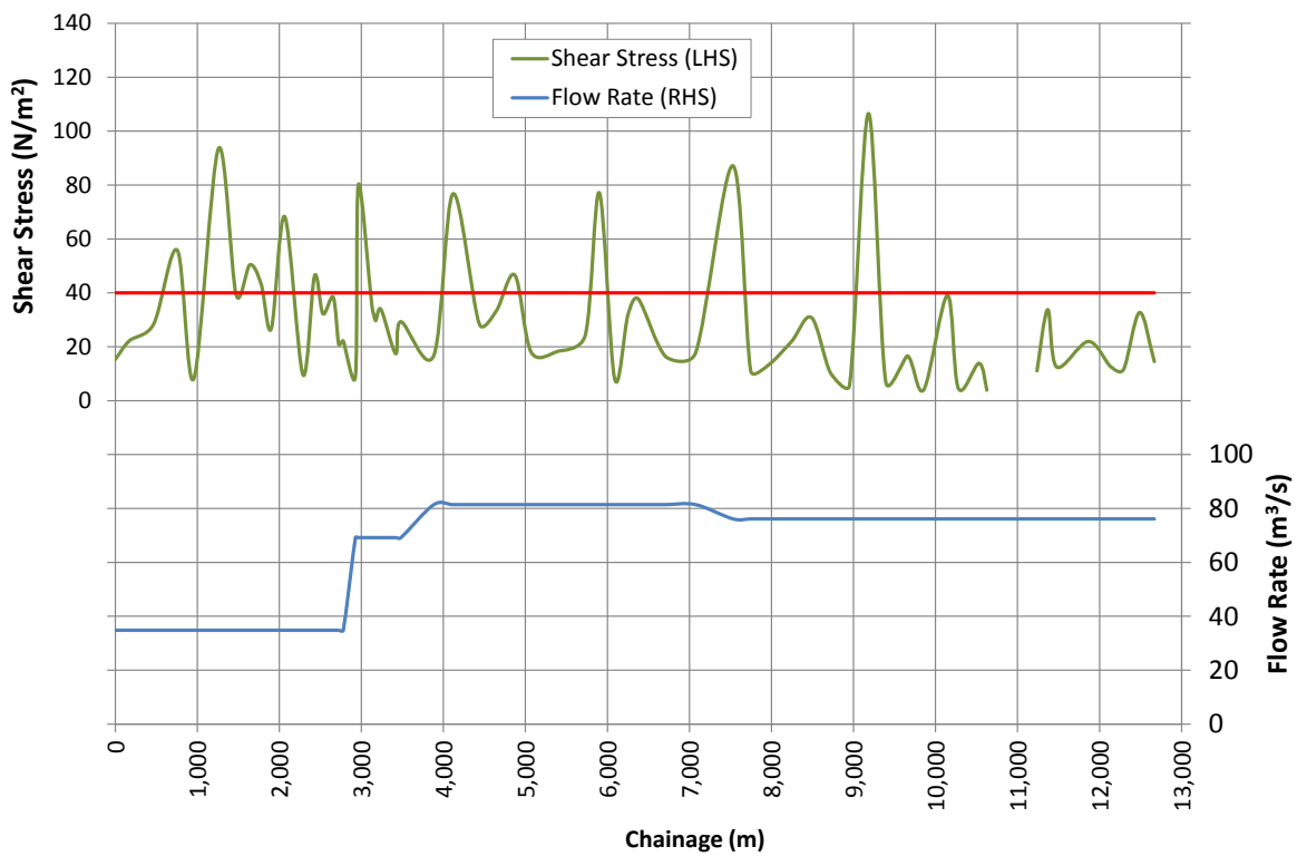
Figure 4-14 Dead Horse Creek Post Development, 2 Year ARI Flow Rate and Shear Stress Variations
