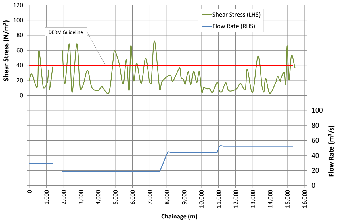
Figure 4-10 Sapling Creek Post Development, 2 Year ARI Flow Rate and Shear Stress Variations
